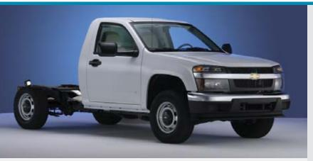
Chevrolet Colorado Chassis Cab gives commercial truck buyers a solid platform to meet their vocational needs. Instead of a pickup box, the chassis cab model allows specific boxes or platforms to be installed by a third-party source.
