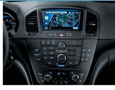
Regal offers an available Navigation<sup>11</sup> Radio that has a 40GB hard drive, uses a multifunction controller on the console and can play AM, FM, XM® CD, DVD and MP3.
