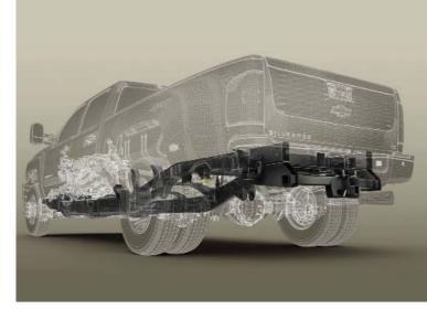
Confident trailering, on single-rear-wheel models, is helped with StabiliTrak and a new Trailer Sway Control (SRW models only) that senses trailer sway and automatically applies the truck's brakes and reduces engine power.
