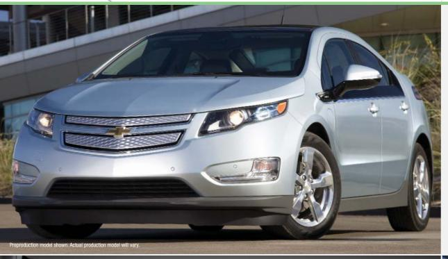
The Chevrolet Volt is an electric vehicle with extended-range capability. It is designed to drive up to 40 miles (assumes fully charged battery) on electricity without using gasoline or producing tailpipe emissions. When the Volt's lithium-ion battery is depleted, an engine/generator seamlessly operates to extend the total driving range to about 300 miles. Production begins late this year.
