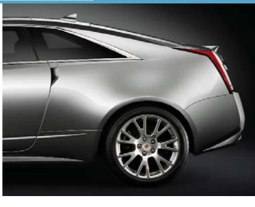
The CTS Coupe offers classic hardtop styling with no conventional B-pillar. Touch-pad operation for the doors removes the need for conventional door handles, creating a technical, clean profile.
