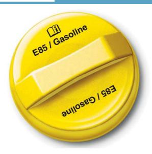
Impala's standard V6 engines have E85 FlexFuel capability that allows the vehicle to run on either gasoline or E85 — a blend of 85% ethanol and 15% gasoline or a combination of both. E85 is a cleaner-burning, mostly renewable fuel source that can be made from U.S.-grown organic materials. It helps reduce greenhouse gases and can enhance the nation's economy and energy independence. Visit gm.com/biofuels to see if there is an E85 station near you.
