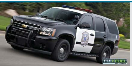
Chevrolet Tahoe Police (PPV) model is only available in 2-wheel drive and has been designed for police work up to and including high-speed emergency vehicle operations. This vehicle is ideal for Standard Patrol, HAZMAT, K9, Medical First Responder and Tactical Operations.
