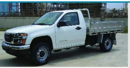
GMC Canyon Chassis Cab gives commercial truck buyers a solid platform to meet their vocational needs. Instead of a pickup box, the chassis cab model allows specific boxes or platforms to be installed by a third-party source.
