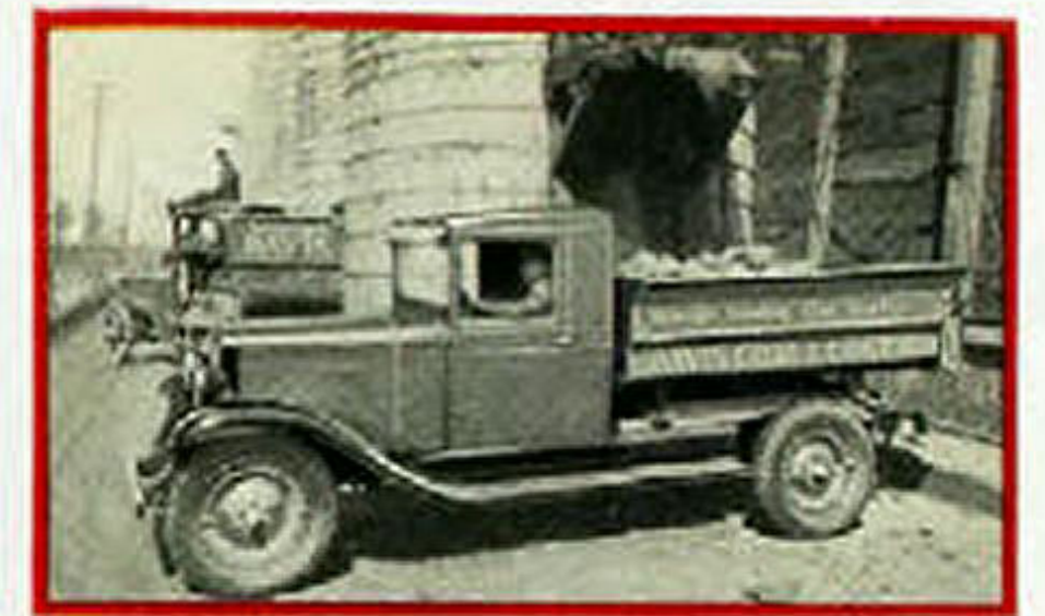
Built of heavy steel to withstand the pressure of concentrated weight, this hand dump body is widely used by coal dealers. Equipped with swinging center partition to divide the load. Coal chute end-gate. Capacity, 1½ cubic yards.
