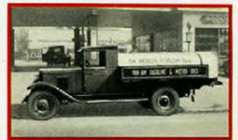
This 400-gallon tank body is widely popular among fuel oil companies. Tank is divided into three compartments. Long side rack for oil containers. Unusually sturdy construction. Also available with glass lined interiors.
