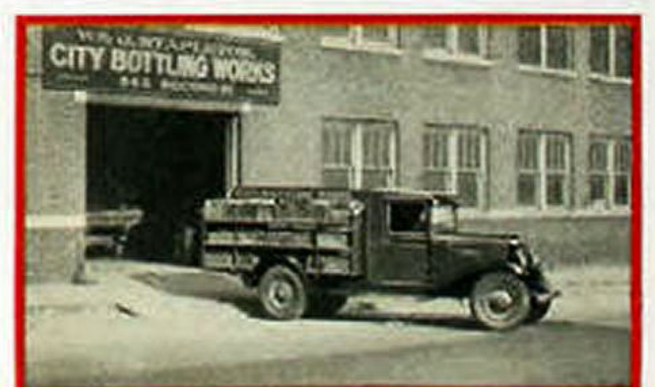
The Chevrolet Utility Truck is a great favorite with bottlers. Shown above is the popular all-steel, three-deck rack for transporting cased bottled goods. Unusually low center of gravity—an important factor in transporting liquids.
