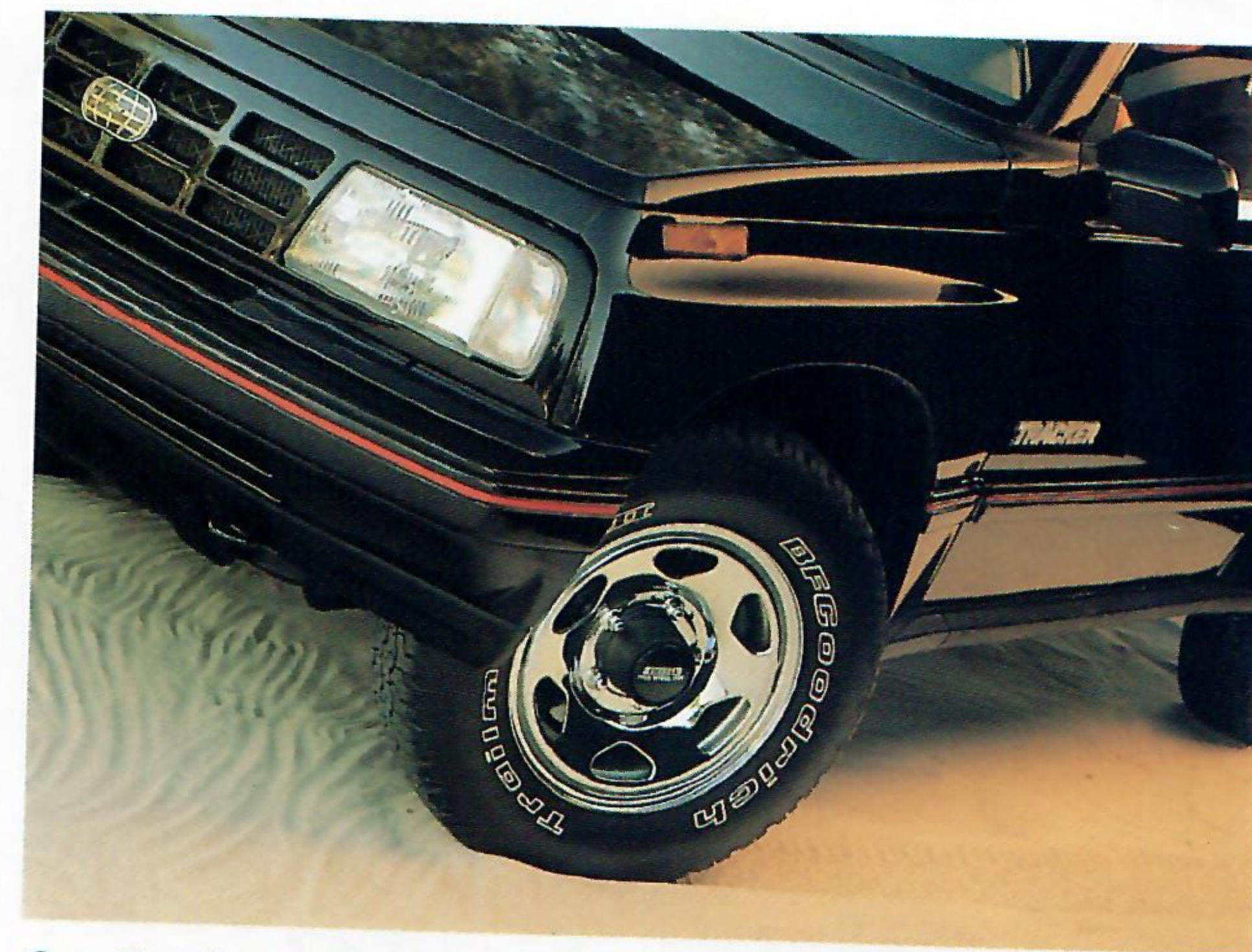
Geo Tracker models feature four-wheel drive with manually locking hubs (automatic locking hubs on Geo Tracker LSi) for selection of 2WD or 4x4 operating modes. The console-mounted transfer case shift lever allows selection of 4-Low or 4-High gear ratios.
