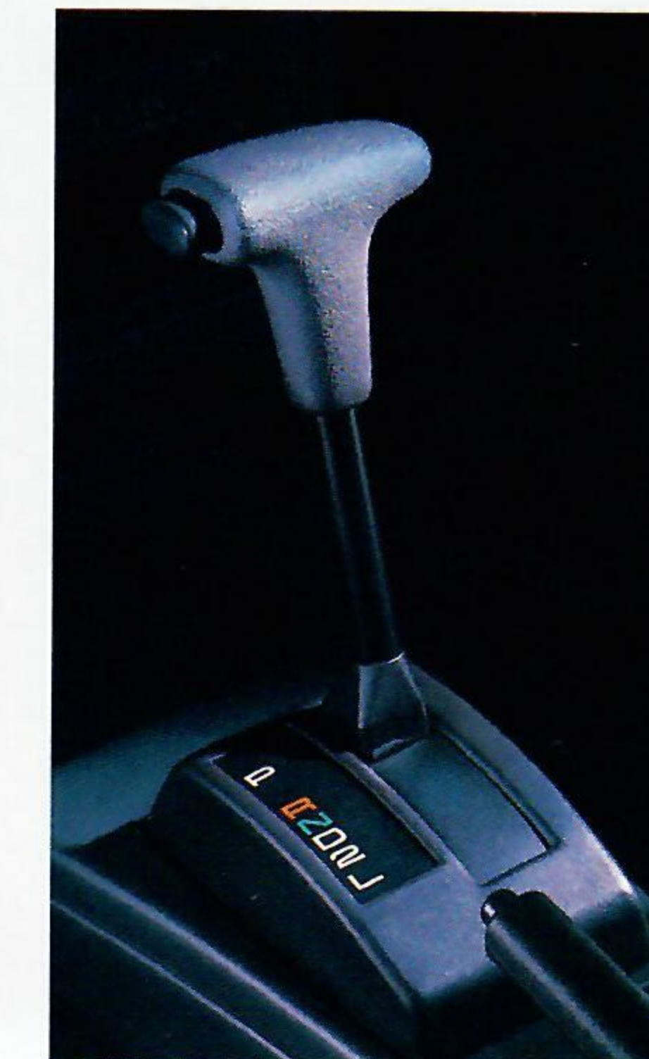
Optional automatic transmission (3-speed on Geo Prizm and Geo Prizm LSi; 4-speed overdrive on Geo Prizm GSi).
