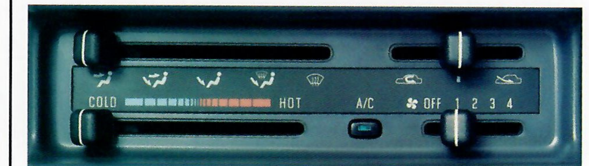
Geo Storm's high-output optional air conditioning features four adjustable instrument-panel outlets, a lap cooler air outlet and 4-speed fan blower. Controls are illuminated for excellent nighttime legibility.
