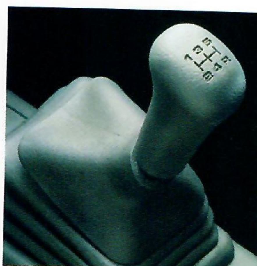
The smooth-shifting 5-speed manual transmission offers 4th and 5th gear overdrive for low-RPM highway cruising.
