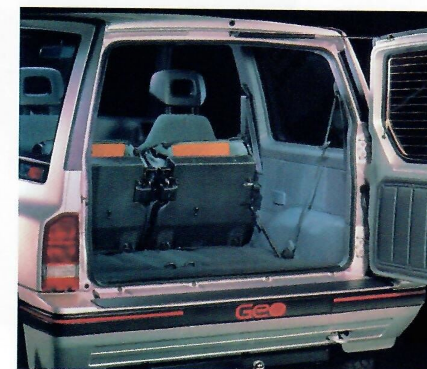
Geo Tracker features a side-opening rear door with glass rear window and electric window defogger.
