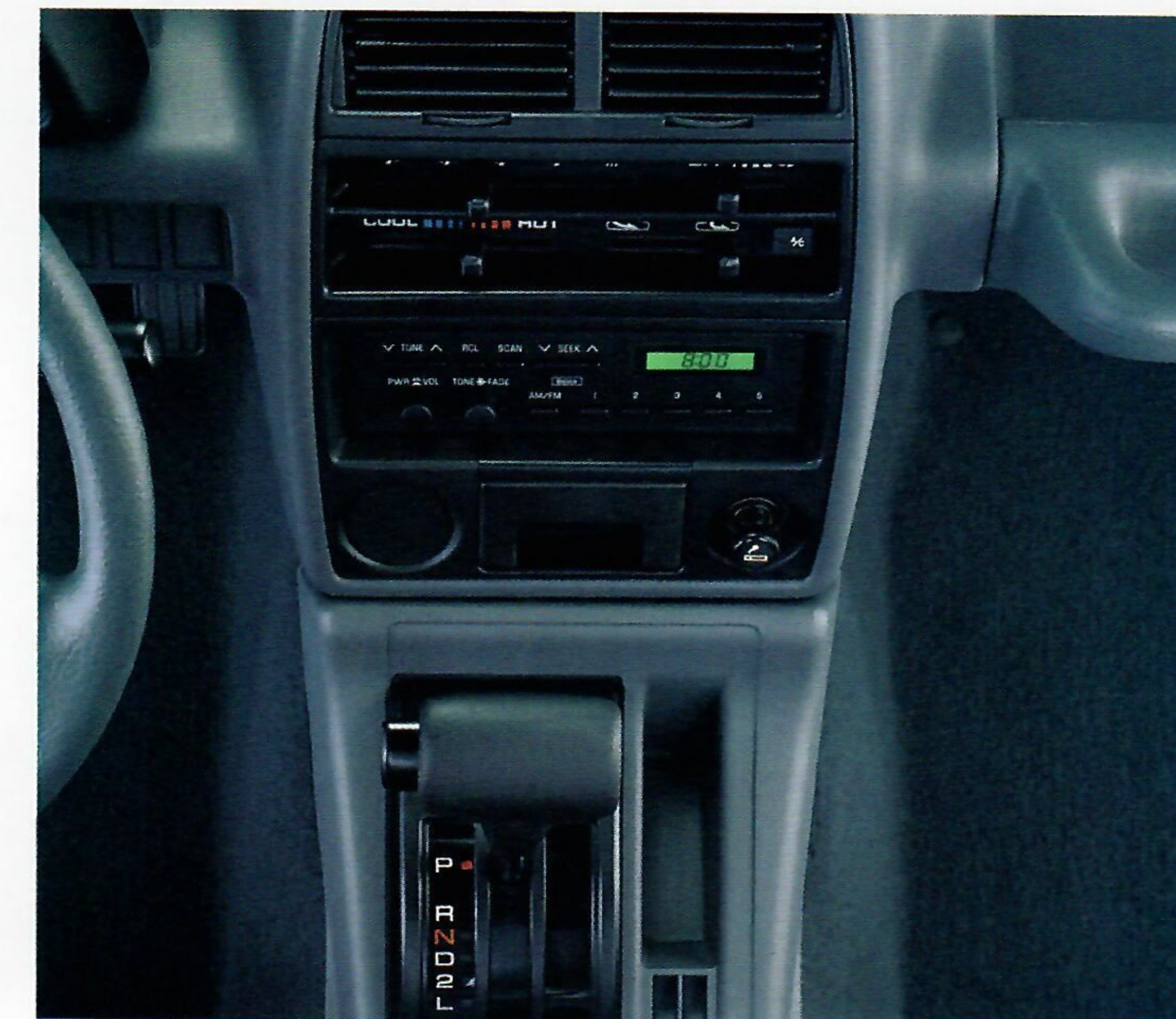
Geo Tracker's center console is attractive and functional. Standard features shown include heater/defroster with power ventilation and 4-speed fan, coin storage, cigarette lighter and ashtray. Optional automatic transmission and AM/FM stereo shown.
