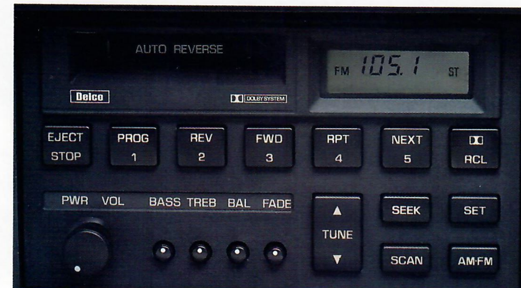
Optional electronically tuned AM/FM stereo with seek-scan, stereo cassette tape player with auto-reverse feature and digital clock.
