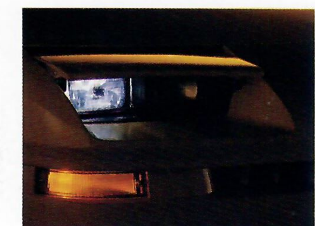
Headlamp covers contribute to Geo Storm's sleek aerodynamic profile. They pop up on demand, revealing quad halogen headlamps.
