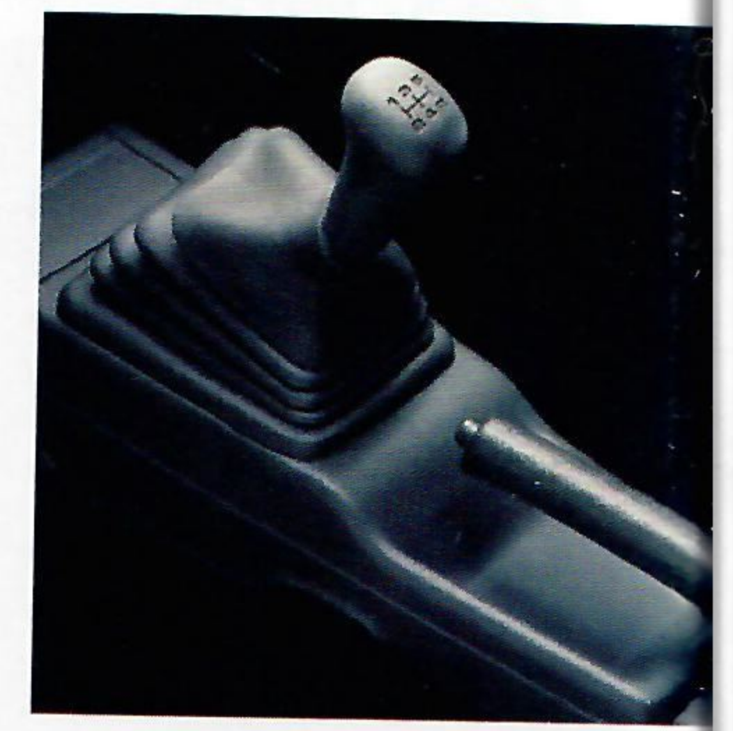
The smooth-shifting 5-speed manual transmission offers 4th and 5th gear overdrive for low-RPM highway cruising.
