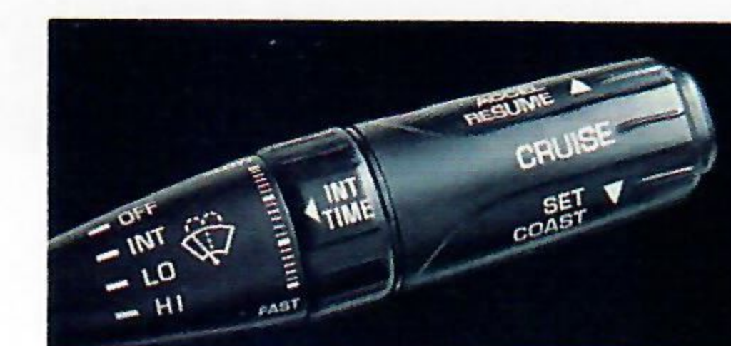
Optional electronic speed control and intermittent wipers add convenience. Controls are stalk-mounted.
