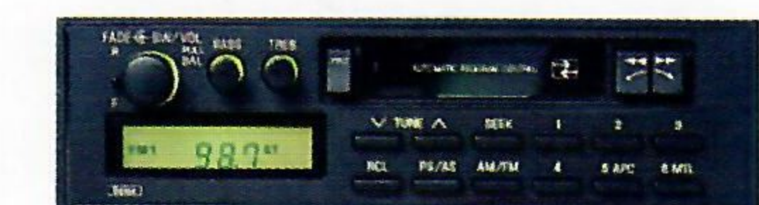
Optional electronically tuned AM/FM stereo with seek-scan, stereo cassette tape player and digital clock.
