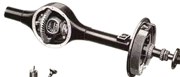
The full floating rear axle—advanced in design—is of the special bevel gear type with straddle mounted pinion. The rugged steel housing, with two large tapered roller bearings in each wheel, carries the rear weight of chassis, body and load.
