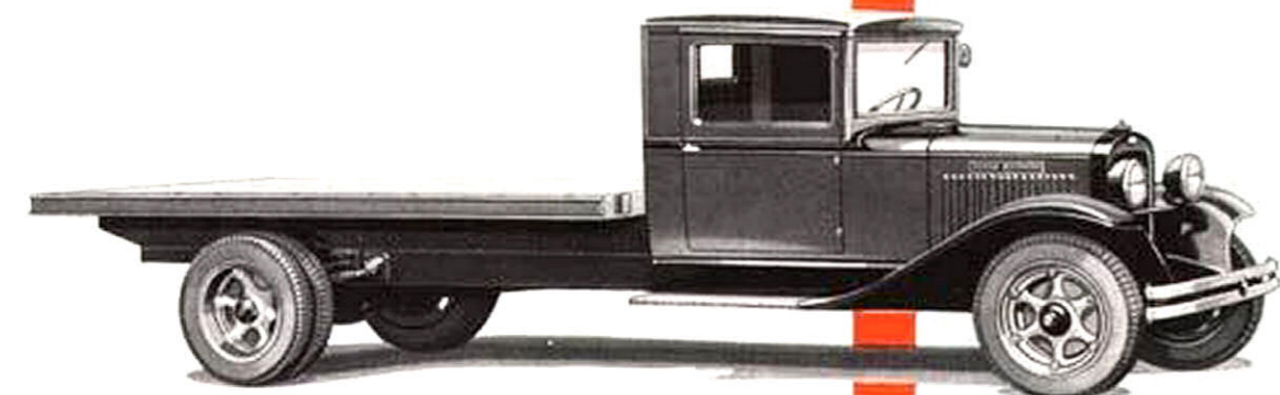
Platform body PUF-31 and Cab ZF-30 mounted on Chassis UF-31D. Loading space: 146¼ inches long, 78 inches wide.
