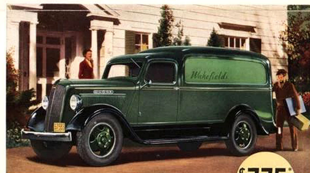
DODGE PANEL, 1 1/2-TON—6 cylinder, 136-inch wheelbase. The smartest looking delivery truck in America. The roomy truck that department stores, fine grocers, etc., have been looking for, with its advanced lines and money-saving features. Inside dimensions: length (on floor from bottom of driver's seat to rear door), 115 1/2 inches; clear loading space, 109 1/2 inches; width between wheelhoists, 48 inches; maximum height at center, 53 1/2 inches; rear door opening, 45 1/2 inches wide, 42 1/2 inches high....
