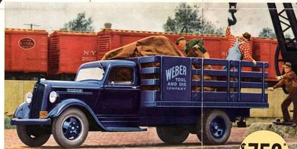
DODGE 12 FT. STAKE, 1 1/2-TON—6 cylinder, built on the 162-inch wheelbase chassis has all famous Dodge features. Body has selected hardwood floor, steel skids channel steel section stakes. Large side board for your advertising sign just behind cab. True streamlined beauty... a handsome and roomy cab with every position for driver comfort and safety. Inside body dimensions: length, 142 1/2 inches; width, 82 1/2 inches; stake height, 40 inches.
