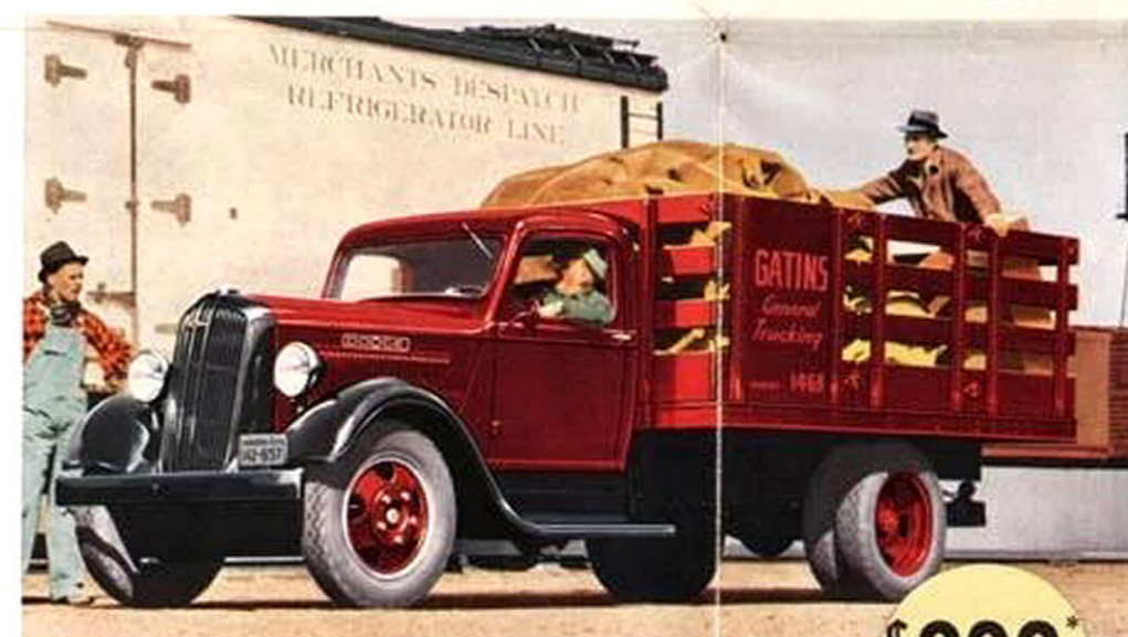
DODGE 8-FT. STAKE, 1 1/2-TON—6 cylinder, 136-inch wheelbase. Packed with famous Dodge dependability features to save you money on running and upkeep; built to outlast them all. Especially popular with general haulers, farmers, contractors. Powerful and flexible. End stakes on front gate have been set closer to center of body to provide space for loading lengths of pipe or lumber along side of cab. Inside body dimensions: length, 106 1/2 inches; width, 82 1/2 inches; stake height, 40 inches....
