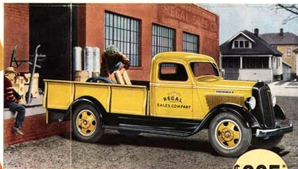
DODGE 1 1/2-TON EXPRESS—6 cylinder, 136-inch wheelbase, smart, sturdy, flexible. Has all famous features that give Dodge "Pre-Proved" Economy. Extra roomy body, rugged construction, ideal for plumbers, steamfitters, electrical contractors and many other truck users. Inside body dimensions: length, 108 1/2 inches; width, 47 1/2 inches; height side panels, 14 1/2 inches; height from floor to top of flareboard, 17 inches.
