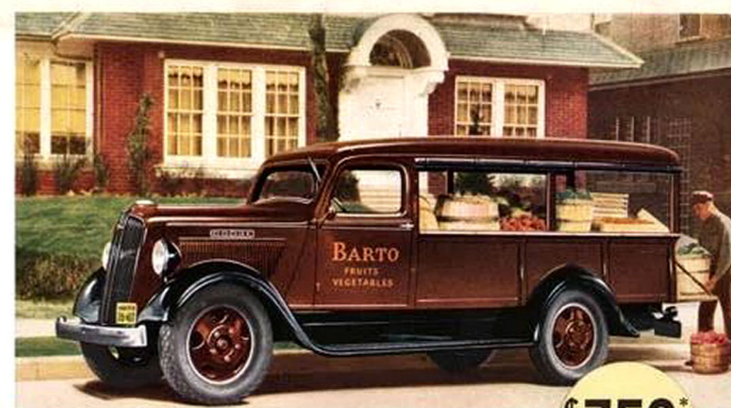
DODGE CANOPY, 1 1/2-TON—6 cylinder, 136-inch wheelbase. A fast, easy-to-handle truck with famous Dodge "Pre-Proved" Economy features, hydraulic brakes and other high-priced truck advantages. Dependable delivery at low cost for meat dealers, grocery houses, produce firms and others. Dimensions of loading space: length on floor, 116 1/2 inches; clear length, 112 1/2 inches; width, 47 1/2 inches; height, 47 1/2 inches. Also available with screen sides at slight extra cost.
