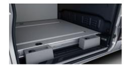
Pallet bracing and tie-downs help when hauling cargo with unusual sizes and shapes34
