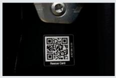
With **RESCUE ASSIST**, SM first responders to an accident can scan a QR code in a Mercedes-Benz Van to quickly see where batteries, airbags, and other structural elements are located in order to safely perform the rescue.
