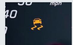
LOAD-ADAPTIVE ELECTRONIC STABILITY PROGRAM (ESP®)<sup>8</sup> This dynamic handling system actively intervenes to help keep the van firmly under control and safe by automatically braking individual wheels and reducing engine power to help stabilize the vehicle if wheelspin, understeer, or oversteer is detected.
