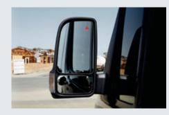
BLIND SPOT ASSIST<sup>3</sup> has Rear Cross-Traffic Alert (RCTA)<sup>4</sup>, which employs automatic braking to avoid a collision with traffic crossing the vehicle's path (e.g., vehicles or pedestrians) when reversing.
