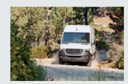
HILL START ASSIST briefly stops the vehicle from rolling backward or forward, giving you an extra level of safety and confidence when making a hill start. Hill Start Assist maintains brake pressure for approximately two seconds, so you can remove your foot from the brake pedal without rolling.
