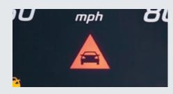
**ACTIVE BRAKE ASSIST**<sup>1</sup> This advanced system senses the likelihood of a collision with a vehicle ahead and sends both a visual and audible warning followed by initiating autonomous braking.
