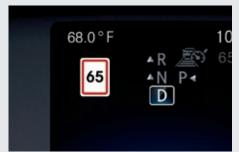
**TRAFFIC SIGN ASSIST**<sup>40</sup> uses a camera to give drivers additional help with identifying speed restriction signs, No Passing zones, and No Entry signs.
