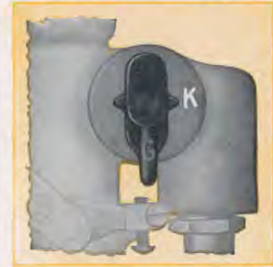
Shifter Valve on Kerosene—Plate No. 16
