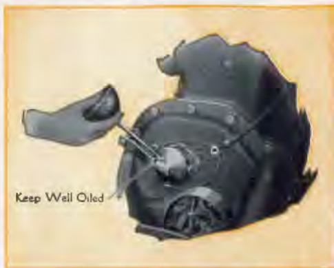
Oiling the Commutator—Plate No. 38
