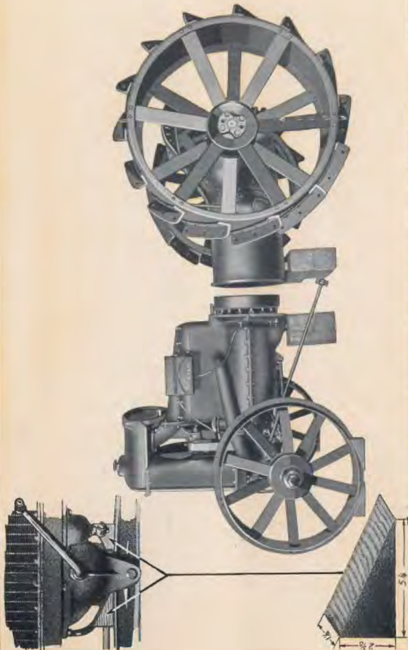
Separating Motor from Transmission—Plate No. 11
