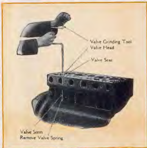
Method of Grinding Valve—Plate No. 9
