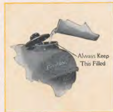
Filling Radiator—Plate No. 13
