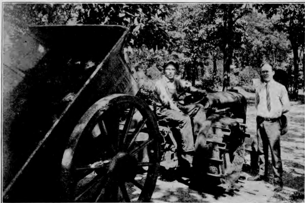
Fordson Operating With Single Dump Cart Under the Trees of Mount Olive Cemetery, Chicago. Note the extension cleats combined with rubber tires on the drive wheels of the Fordson. Man standing is Charles A. Palm, assistant to the superintendent; operator of the Fordson is William A. Veach
