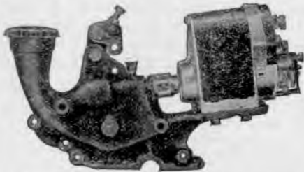
Fits on in place of Ford timing gear cover.
