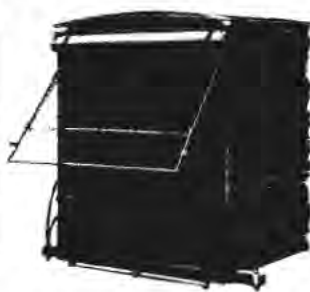
No. 73 Rear—Tail Gate, Curtain and Hinged Screen for Bodies 220 and 320. No. 74 Rear—same for Body 120. Furnished at extra cost in place of rear doors.
