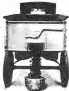
View of coal chute endgate—No. 3003—for dumping coal in basket or basement.
