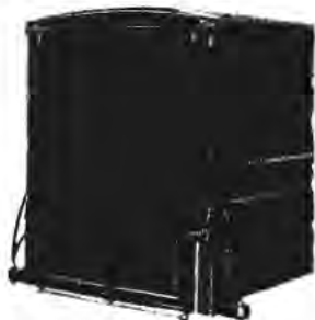
No. 71 Rear—Tail Gate and Curtains for Bodies 220 and 320. No. 72 Rear—same for Body 120. Optional, in place of rear doors.
