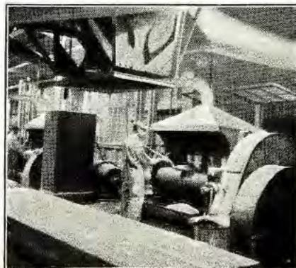
Rubber Compound Is Kneaded Here
