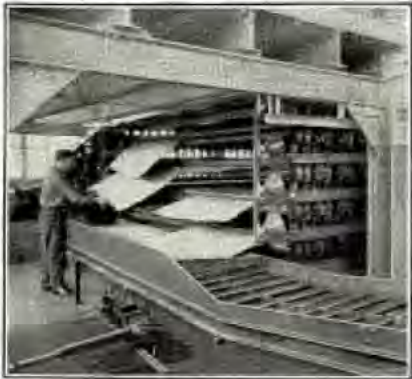
Paper Comes in Large Wet Sheets. Drying is Done in Long Ovens.
