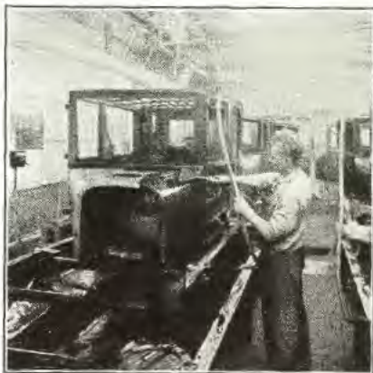
Painting Bodies by the Gravity Flow Method.
