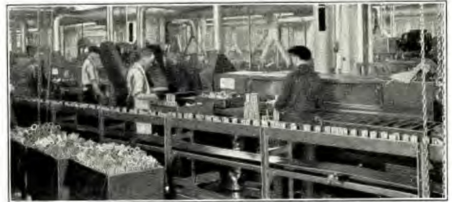
Bearings Conveyed Away After Final Inspection
