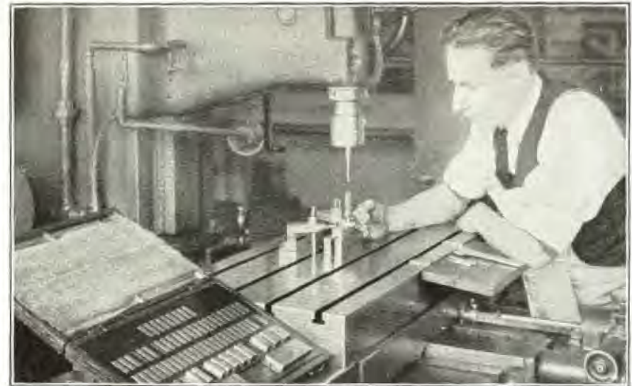
Adjusting a Machine with the Aid of Johansson Gage Blocks.
