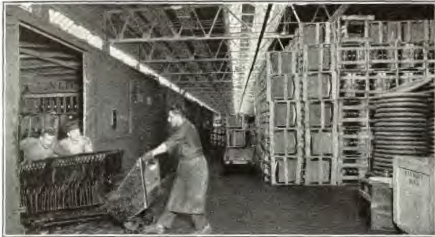
Receiving Knocked Down Parts at an Assembly Plant—In the Newer Plants the Longest Trucking Distance is 20 Feet
