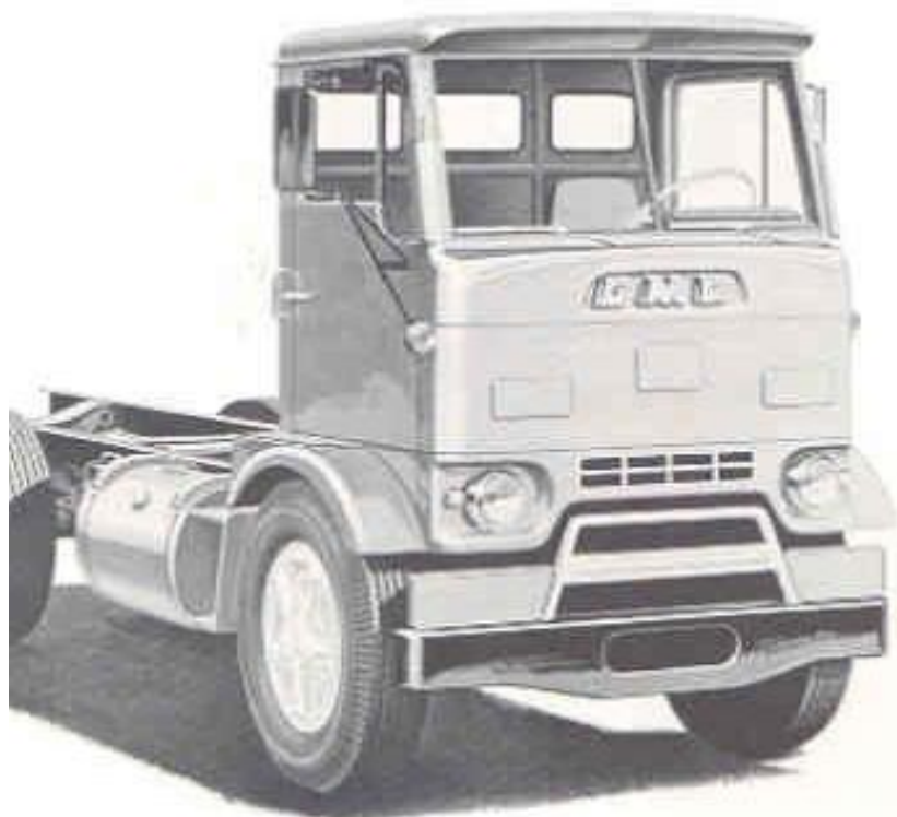
Facing lamp, fuel tank and rear side window shown are optional at extra cost.
