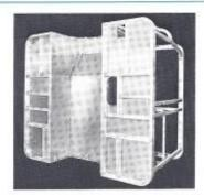
ENGINE COVER AND FLOOR STRUC-TURE — Lightweight, strong .100" thick aluminum forms the engine cover and the floor structure. The aluminum substructure is constructed of aluminum channel that is slip fitted and securely welded.
