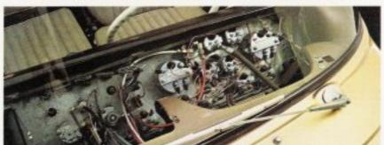
A TILT-AWAY STEERING COLUMN AND AN INSTRUMENT PANEL THAT FOLDS COMPLETELY DOWN. Just lower the steering column, swing the instrument panel down, and you have complete pillar-to-pillar access to electrical connections, tubing, valves, and instruments. The steering column also adjusts to the height the driver finds most comfortable.
