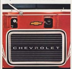
Twin access doors for easy servicing. Front service access panels allow checking and topping off of lubricant and coolant as needed with the cab in the down position. Radiator sight glass facilitates fast checks of coolant level.
