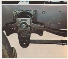
Reyco 101 tandem suspension. The weight-saving steel leaf-spring Reyco 101 tandem suspension, rated at 34,000 pounds, is available.
