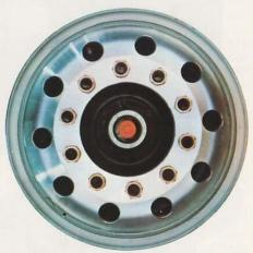
Lightweight wheels. Strong, polished aluminum disc front wheels are available on the Titan-Lite, along with high-tensile steel rear wheels
