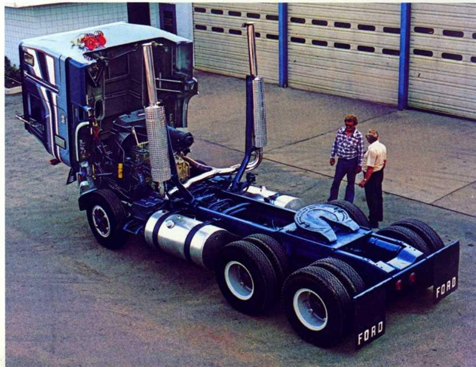
Cab tilts by manual hydraulic pump or optional air pump.
