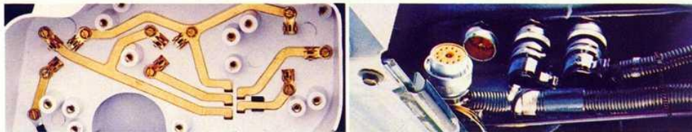
Bus bars replace many wires to instruments.
