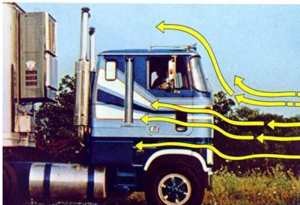
Air flows smoothly around the aerodynamic cab.
