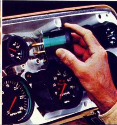
Gauges and switches are all plug-in type.
