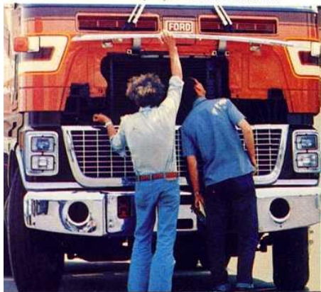
Grille lifts for service checks.
