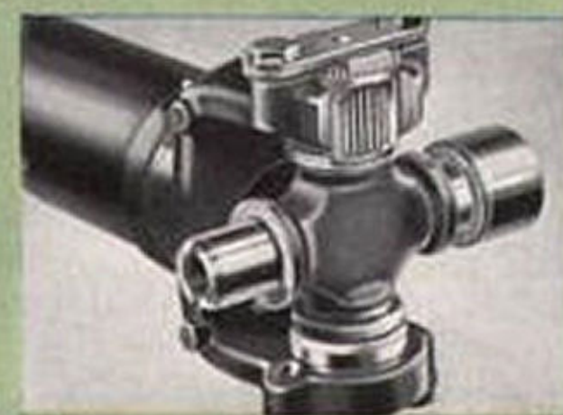
ROLLER-BEARING UNIVERSALS —Pioneered by Dodge in low-price trucks. Reduces friction and wear. Sealed against dust and water or loss of lubricant.
