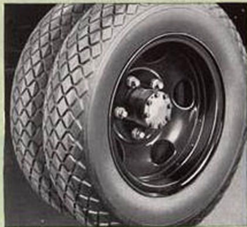
NEW REAR WHEEL HUBS PERMIT EASY INTERCHANGE OF DUAL OR SINGLE REAR WHEELS INTERCHANGEABLE DUAL WHEELS —Single or dual wheels without need for special hubs (excepting on 1 1/2-Ton Express). Easy change-over simply by taking off or putting on outside wheel. Generous chain clearance on all models.
