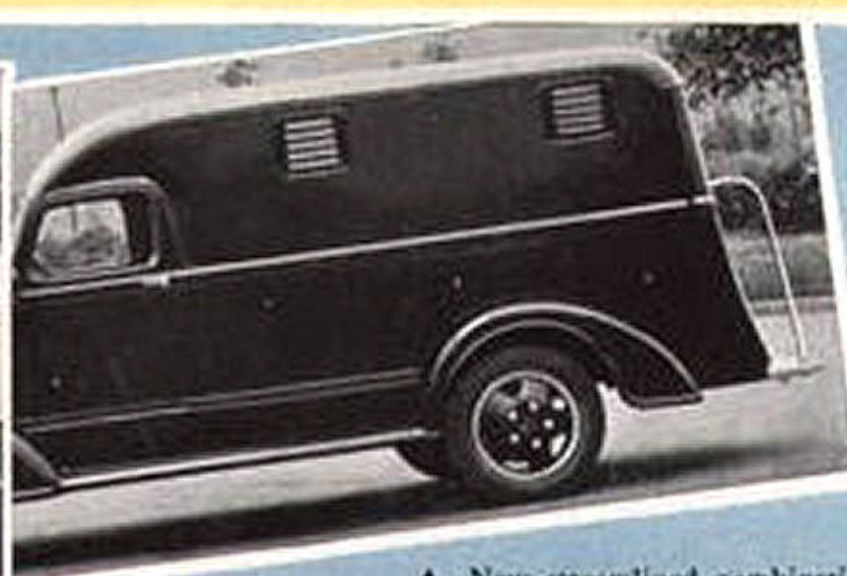
▲ New streamlined combination police patrol and ambulance body factory mounted on 1 1/2-Ton, 133" Dodge truck chassis.
