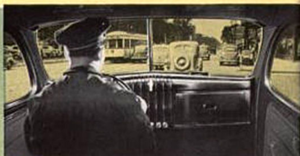
BETTER VISION, BETTER VENTILATION Wider, higher V-type windshield that opens plus wide cowl ventilator for maximum air circulation through cab. Defroster vents at windshield may be coupled with a heater for winter driving safety. Note higher driver seat position, high, broad door windows, narrow corner pillars, new-style instrument panel, extra-large package compartment.
