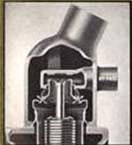
DODGE BY-PASS THERMOSTAT —Makes engine warm up quickly. Eliminates localized hot spots and cylinder distortion.
