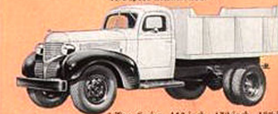
3-Ton Series, 152-inch, 170-inch, 188-inch, 205-inch wheelbases. Five-speed transmission.
