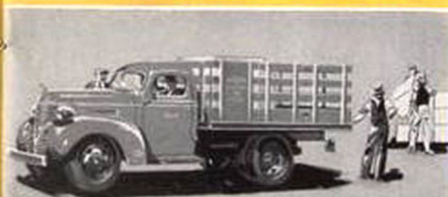
135" W.B. 1 1/2-Ton Heavy Duty Stake Body 106 1/2" x 82" (inside.)
