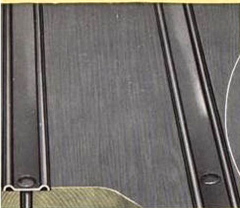
STAKE FLOOR —Typical Dodge extra-strength construction includes sturdy steel gusset re-inforcements on body sills, steel stake posts, heavy wood floors re-inforced with broad steel strips.
