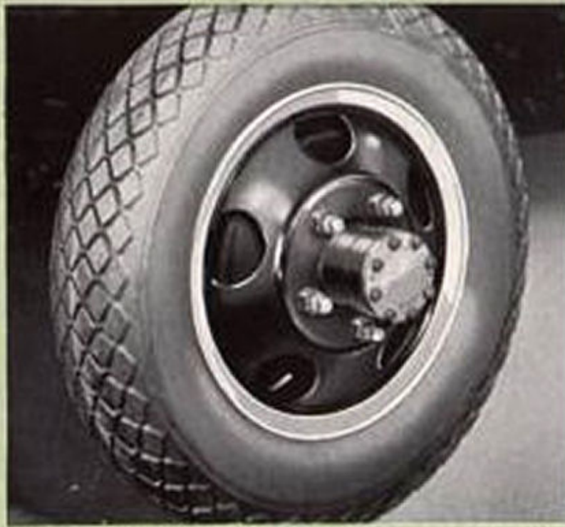
NEW REAR WHEEL HUBS PERMIT EASY INTERCHANGE OF DUAL OR SINGLE REAR WHEELS INTERCHANGEABLE DUAL WHEELS —Single or dual wheels without need for special hubs (excepting on 1 1/2-Ton Express). Easy change-over simply by taking off or putting on outside wheel. Generous chain clearance on all models.
