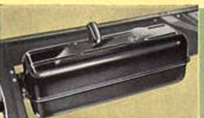
FUEL TANK —Spring-mounted, pressed steel 18-gallon gas tank, permanently welded into one piece.
