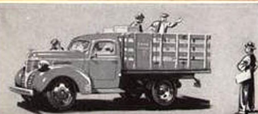
155" W. B. 1 1/2-Ton Standard Stake, Body 106 1/2" x 82" (inside.)
