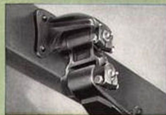
SPRING SHACKLE —New, stronger rear spring shackles in 1939 Dodge trucks. Shackle pins have been increased in diameter giving 16% larger bearing area for longer life.
