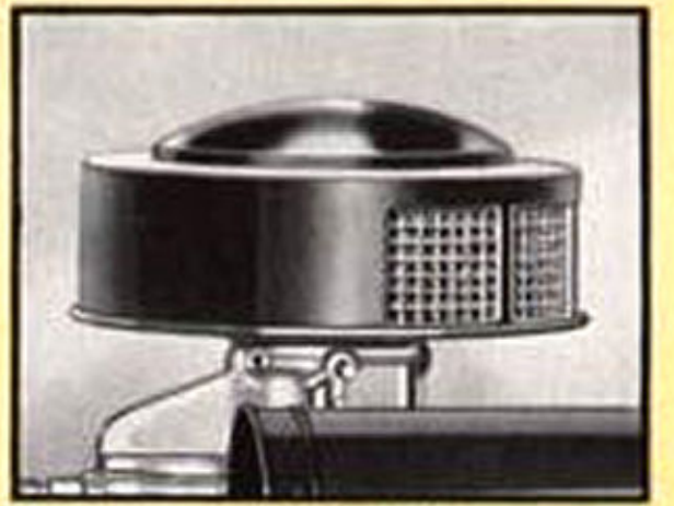
OIL-WETTED AIR CLEANER —Filters all air entering carburetor. Same principle used in large air conditioning systems. Prevents cylinder abrasion commonly caused by road dust and grit.
