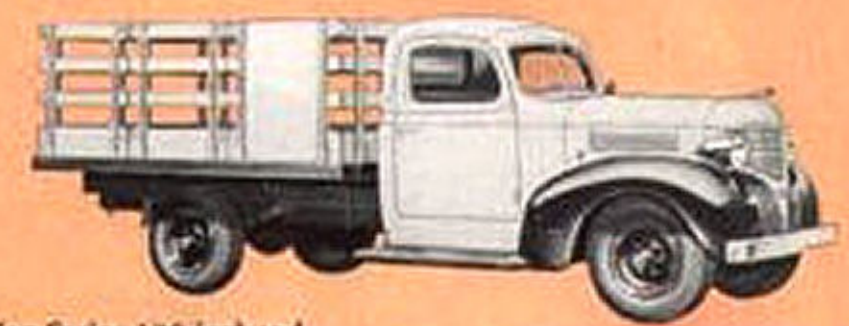
1-Ton Series, 120-inch and 133-inch wheelbases. Six types and sizes of bodies. (Also 1 1/2-Ton Series. Available in 120-inch wheelbase, with three types and sizes of bodies.)
