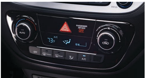
Automatic temperature control
