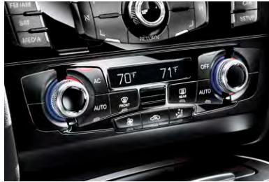
Three-zone automatic climate control
