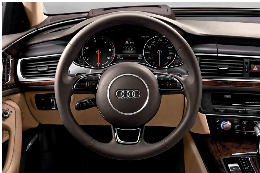
Three-spoke multifunction steering wheel with shift paddles, 7" color driver information system and head-up display
