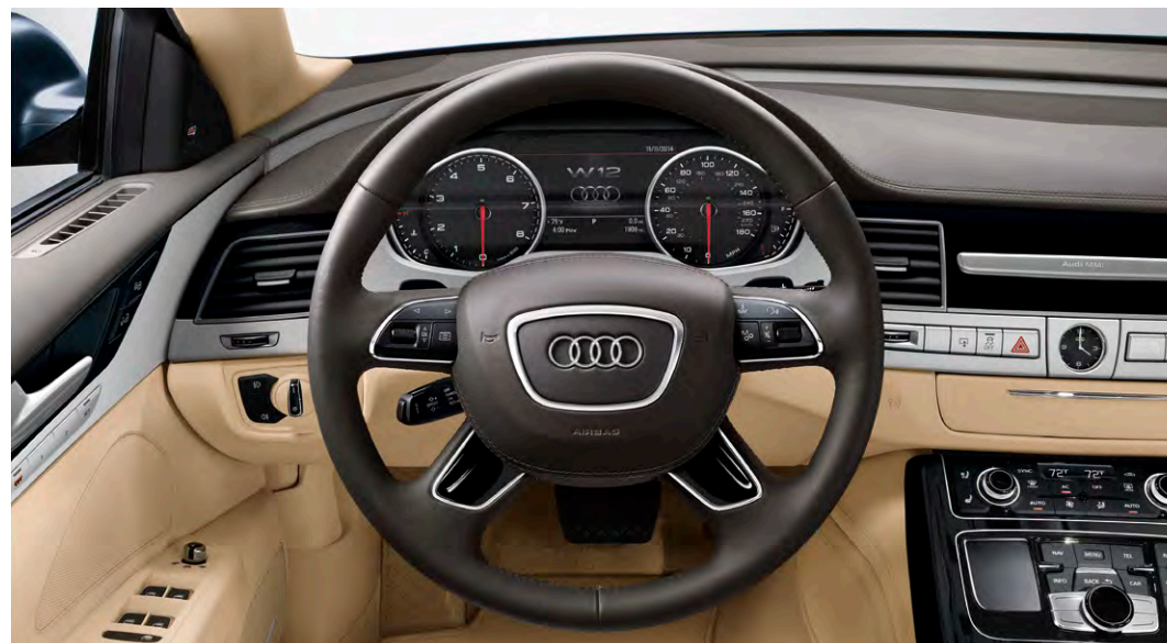
Four-spoke multifunction steering wheel with shift paddles, 7" color driver information system, and head-up display
