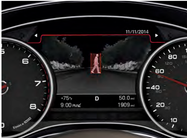
Night vision assistant with pedestrian and large animal detection (optional on all models)
