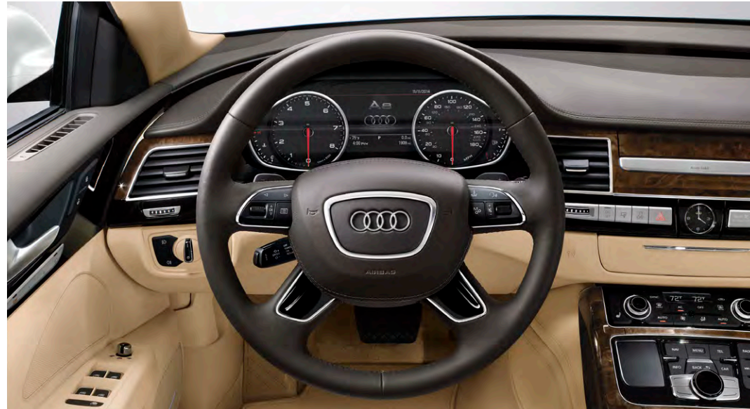
Four-spoke multifunction steering wheel with shift paddles and 7" color driver information system
