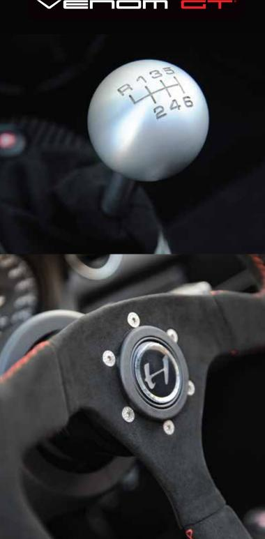
The Venom GT's components and systems are built for purpose, not flash. A lightweight carbon-fiber console surrounds an alloy shifter that actuates a Ricardo 6-speed manual gearbox.
