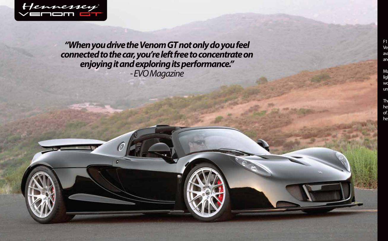
F1 meets road car. To maximize the power-to-weight ratio, the Venom GT utilizes some of the most high-tech racing components available today. This includes the use of carbon-fiber body panels and lightweight forged aluminum monoblock wheels.
