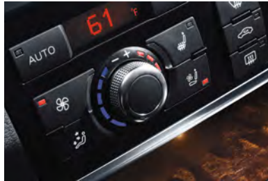
Front seat temperature controls
