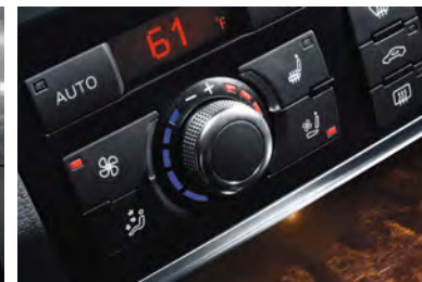
Front seat temperature controls
