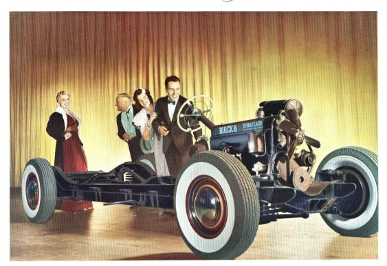
☼ The chassis is the foundation upon which any car is built. Without an exceptional chassis, it is obvious that neither exceptional comfort and steadiness nor exceptional performance can be obtained. Here illustrated is the ruggedness of the Buick Limited chassis, with its nine-inch-deep frames, rigidly cross braced and with full cross section side rails for strength.
