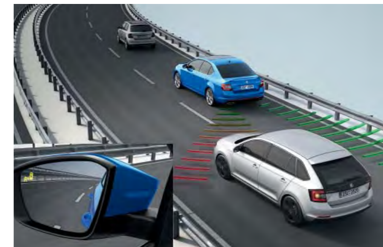
BLIND SPOT DETECT Using radar sensors in the rear bumper, Blind Spot Detect monitors the blind areas behind and beside the car. Based on the distance and speed of the surrounding vehicles, it decides whether or not it should warn the driver.
