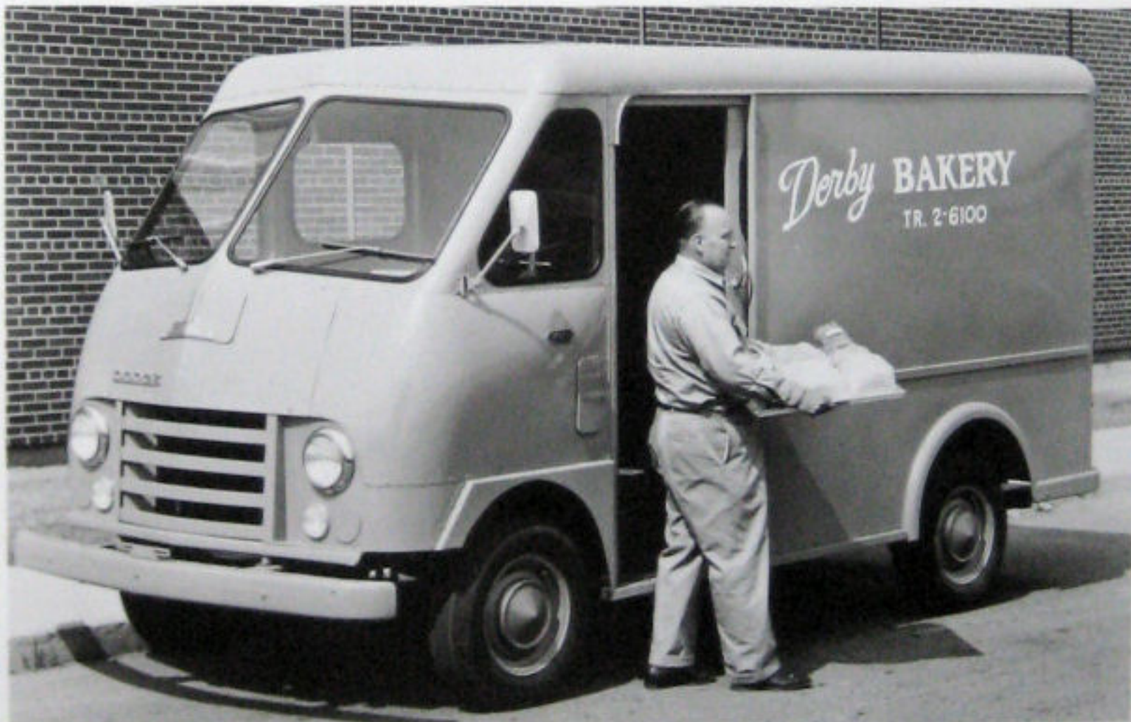
COMPACT DODGE -- Ideal for firms engaged in delivery operations in congested urban areas, this compact 1962 Dodge P-100 forward-control truck provides outstanding maneuverability on a short, 104-inch-wheelbase. A 140-horsepower, Inclined 6-cylinder engine is standard, and a 101-horsepower "Six" is optional. The truck has a maximum gross vehicle weight rating of 5,100 pounds.
