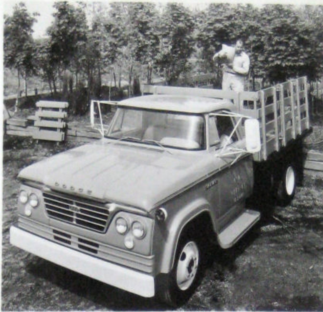
ECONOMICAL STAKE -- Highly maneuverable on a 133-inch-wheelbase, this 1962 Dodge D-300 stake model features a 140-horsepower, Inclined 6-cylinder engine. Standard on the unit, which has a 9-foot body, is a 4-speed transmission. The D-300 has a maximum gross vehicle weight rating of 10,000 pounds.
