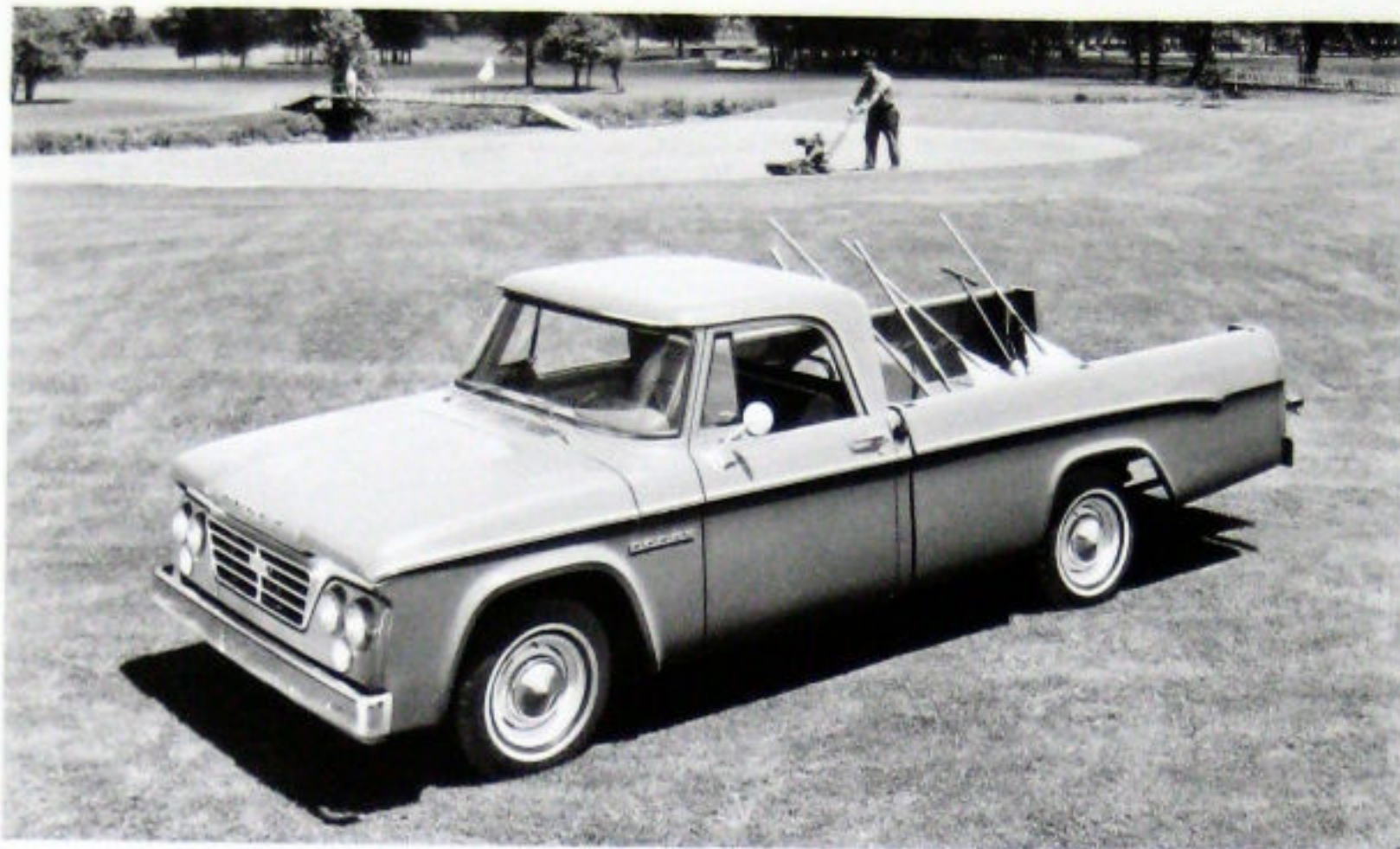
VERSATILE DODGE TRUCK -- At home in the city and on the farm, the 1962 Dodge D-100 Sweptline pick-up features a handsome one-piece chromium-plated steel grille, low hood silhouette and contemporary styling. The Sweptline is powered by a 140-horsepower, 225-cubic-inch, Inclined 6-cylinder engine. It is available with a 6 \frac{1}{2} -foot or 8-foot body. Its maximum gross vehicle weight rating is 5,100 pounds.
