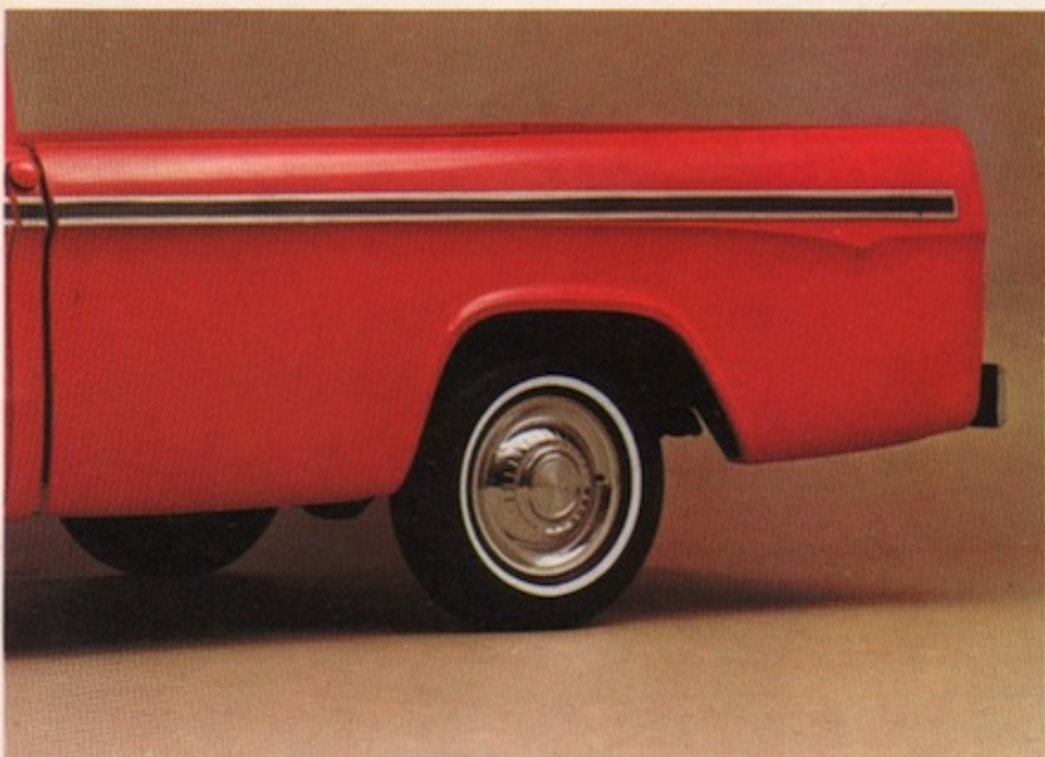
ONE-PIECE OUTER SKIN WITH NO RUST-COLLECTING POCKETS
