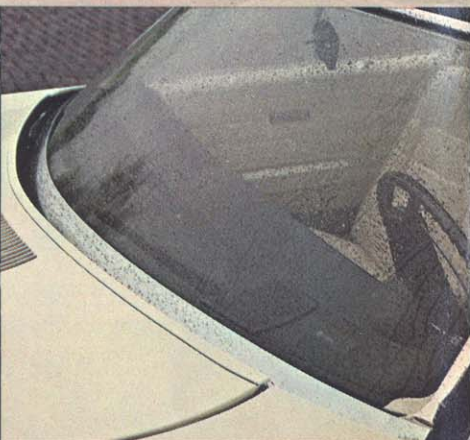
Concealed windshield wipers—tuck away when not in use
