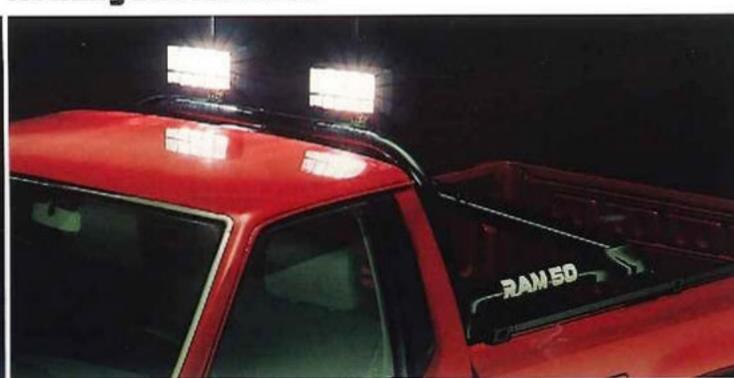
Light Bar and Off-Road Lights: The sturdy light bar makes a firm foundation for these bright halogen lights, which feature mirror reflectors and integral lens guards. (Sold separately. See back cover note.)
