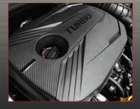
**1.6 L TURBOCHARGED GDI ENGINE** delivers 201-horsepower and up to 195 lb.-ft. of torque
