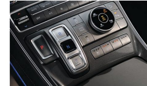
Push-button Shift-by-Wire gear selection
