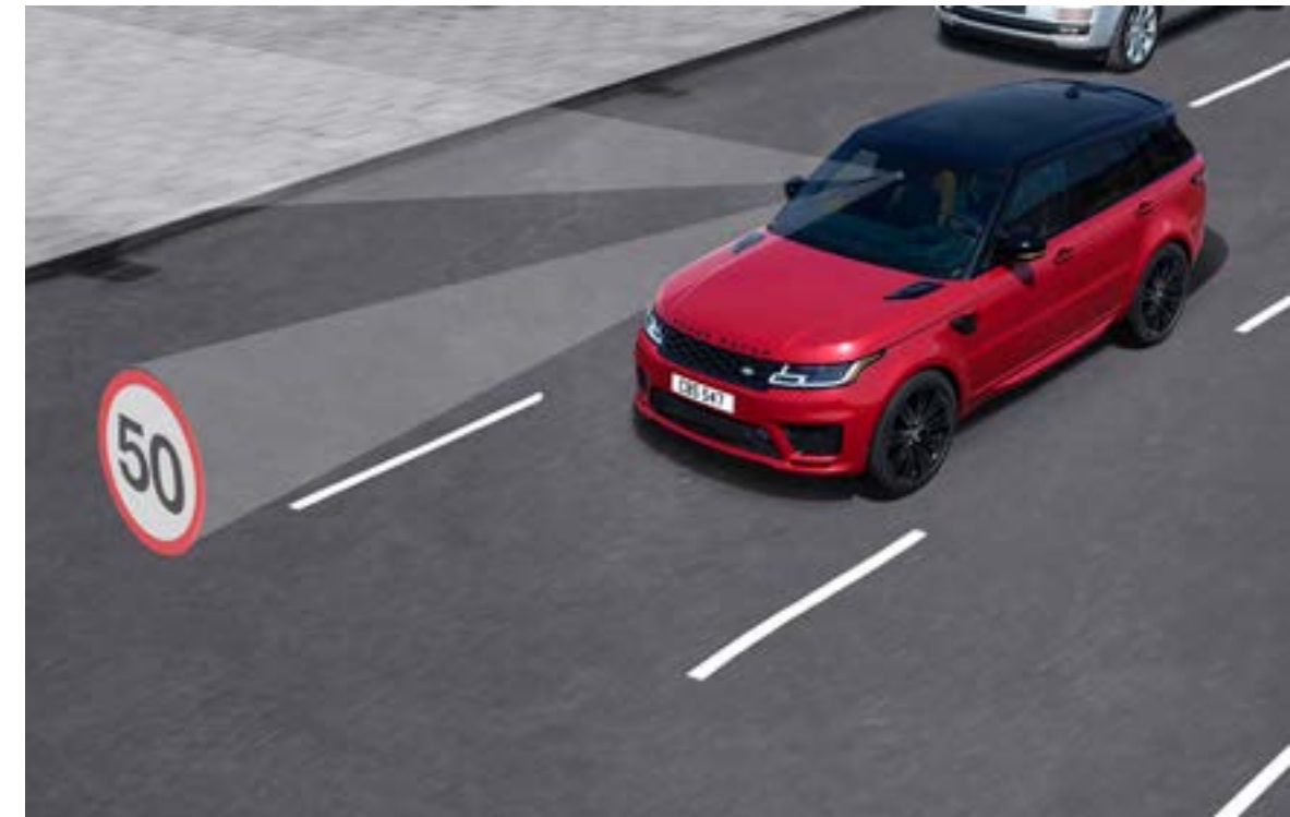
Traffic Sign Recognition with Adaptive Speed Limiter
