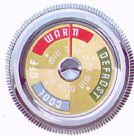
DIAL-TEMP SYSTEM* —One dial tunes in both heating and ventilation and also accommodates optional air conditioning. Automatic controls make all the adjustments.
