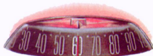
SPEED WARNING LIGHT SPEEDOMETER* —You simply set the rotating warning dial to the safe cruising speed of your choice and when you exceed it, speedometer dial lights up in red.
