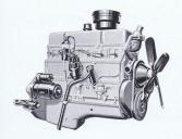
JOBMASTER 6 engine as standard equipment keeps bigger jobs moving for less. With a displacement of 261 cubic inches, its extra-duty features include Stellite-faced exhaust valves equipped with Rotocoils for long life in severe service, full-flow filter to keep oil cleaner, and positive crankcase ventilation to extend engine life.
