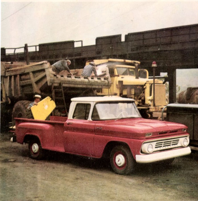
1962 STEPSIDE PICKUPS —Five husky models with convenient side running boards, GVW's from 4,300 to 7,800 lbs., wheelbases of 115, 127 and 133". Bodies up to 108 inches provide ample room for bulky loads. Independent Front Suspension gives a smooth ride that saves on truck wear, cargo damage, and maintenance. High Torque 6-cylinder or V8 engines supply plenty of low-cost power.
