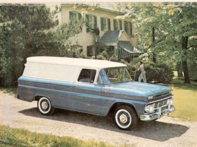
1962 PANELS —Newly styled, sturdy-built and spacious, three big panel models for '62 offer up to 231 cubic feet of cargo with GVW ratings as high as 7,800 lbs. For economical, dependable power, Chevy's famous High Torque 235 Six-cylinder engine is standard; also, the hard-working High Torque 261 Six and 283 V8 are optional at extra cost. High, wide rear doors and low floor height ease loading.
