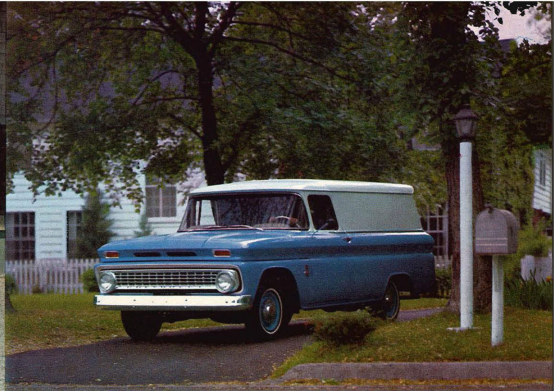
Panel models —Here to handle big loads with ease and efficiency, Chevrolet's 3 new panel models range in GVW's from 4,100 to 7,800 lbs.; carry up to 3,300 lbs. of cargo smoothly with new work-tested independent front suspension with coil springs and new two-stage rear coil springs as standard equipment. Bodies in 7 \frac{1}{2} '- and 10 \frac{1}{2} '-foot lengths.
