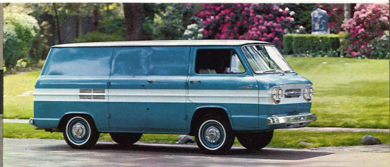
Panel models —Here to handle big loads with ease and efficiency, Chevrolet's 3 new panel models range in GVW's from 4,100 to 7,800 lbs.; carry up to 3,300 lbs. of cargo smoothly with new work-tested independent front suspension with coil springs and new two-stage rear coil springs as standard equipment. Bodies in 7 \frac{1}{2} '- and 10 \frac{1}{2} '-foot lengths.
