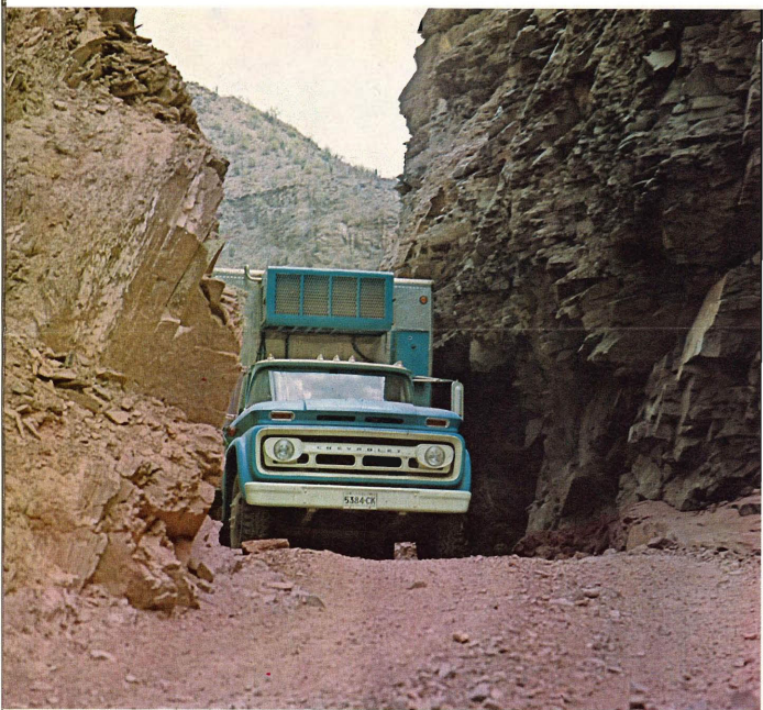
Grueling travel in the canyon country (southern Baja) illustrates an advantage of Chevy's new trim-line design. Medium- and heavy-duty trucks, with new sheet metal contours that reduce truck width by more than 7 inches, were able to work their way through extremely tight cuts in the canyon walls. Series 60 Van pictured here was powered by the new High Torque 232 Six and it performed perfectly throughout the entire run.
