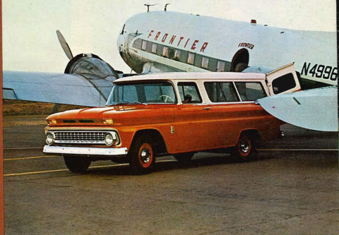
Suburban Carryall —The most versatile of vehicles, the Suburban Carryall combines station wagon styling with true panel truck utility; seats up to 8 passengers or carries up to 1,000 lbs. of cargo with the seats removed. Available with either panel or station wagon type rear loading doors.
