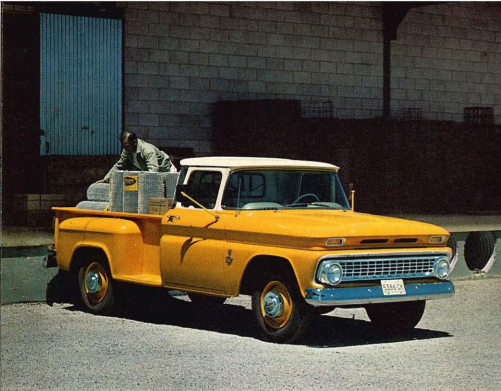
Stepside pickup —Five Stepside models in the \frac{1}{2} -, \frac{3}{4} - and one-ton classes with GVW's from 4,100 to 7,800 lbs. are offered with body lengths ranging from 6 \frac{1}{2} ' to 9 feet. Durable select wood floors with recessed steel skid strips simplify loading. Wide choice of 6-cylinder or V8 power offers top operating economy for any job.
