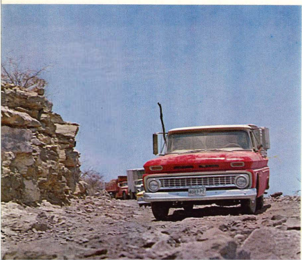
Grueling travel in the canyon country (southern Baja) illustrates an advantage of Chevy's new trim-line design. Medium- and heavy-duty trucks, with new sheet metal contours that reduce truck width by more than 7 inches, were able to work their way through extremely tight cuts in the canyon walls. Series 60 Van pictured here was powered by the new High Torque 232 Six and it performed perfectly throughout the entire run.
