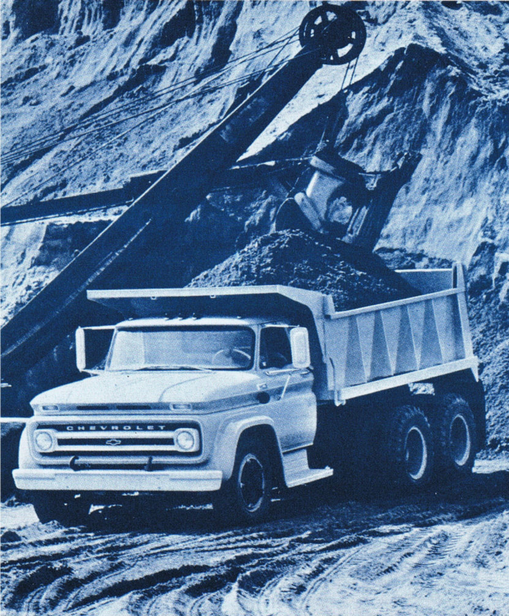
M60 and M80 Series (GVW Rating 30,000 lbs. to 43,000 lbs.) (GCW Rating 35,000 lbs. to 51,000 lbs.)
