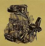
HIGH TORQUE 153 FOUR—Chevyl's High Torque 153 Four brings you the fuel-saving economy of a lightweight space-saving four-cylinder engine. Standard power for the 153 Four delivers 90 hp and 152 ft.-lbs. of torque, ample power for most light-duty loads. With a 3/8/ ×3 1/4 bore and stroke, overhead valve design, hydraulic valve lifters and tough 5-bearing crankshaft, the Chevrolet High Torque 153 Four is a sure saver on any run.
