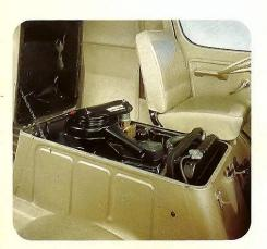
engine compartment is welded to steel floor panel to form a strong, rigid "isolation" chamber around engine at and noise. A hinged lid swings back in a 95-degree and is held in place by a retaining chain for routine service and maintenance work. Engine compartment lid is insulated for minimum transfer of heat and noise.
