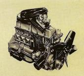
HIGH TORQUE 230-SIX—Now for 1965, Chevy's work-proved 230-Six is available for those delivery jobs that call for the extra power and durability of a big truck engine. Rated at 140 hp and 220 ft. Ibs. of torque, the 230-Six delivers plenty of power for those tough hauls. Such quality features as 7-main bearing crankshaft, replaceable main bearings, hydraulic valve lifters and more help assure long, dependable economical performance.
