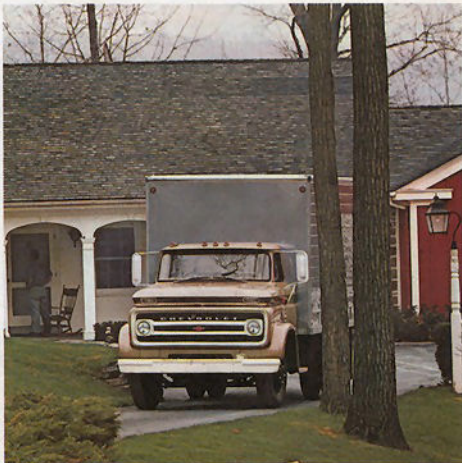
Chassis with LCF 93-inch cabs offered in three series. GVW ratings to 32,000 lbs., GCW ratings to 51,000 pounds. Five wheelbases.
