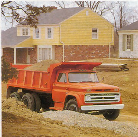
Tandems with conventional cabs are of two types — trailing-axle tandems to 30,000 lbs. GVW and dual-drive tandems to 45,000 lbs.
