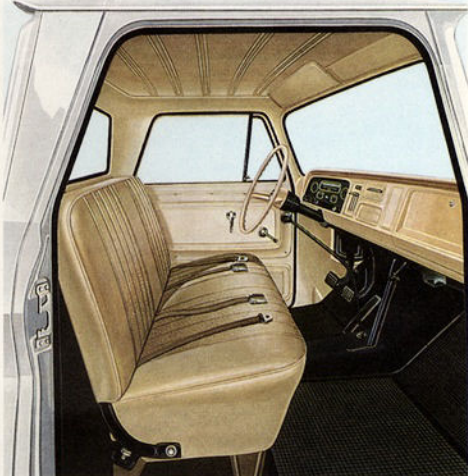
STANDARD CAB —Deep-cushioned seat is upholstered in easy-to-clean vinyl. A full-depth foam seat with vinyl upholstery is also available, as well as an adjustable Bostrom Level-Ride seat.
