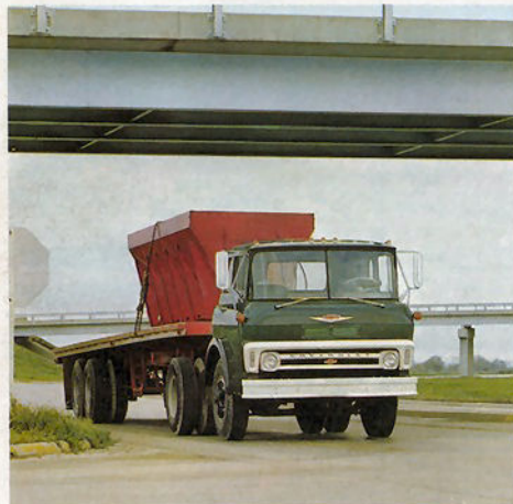
Chassis with short 72-inch tilt cabs offered in three series. GVW ratings to 32,000 lbs., GCW ratings to 51,000 pounds. Five wheelbases.
