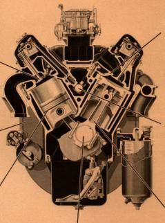
Cylinder heads of highquality alloy cast iron are short and extra rigid with a six-bolt attachment pattern around each cylinder bore for extra-secure sealing. Large freebreathing valve ports and throats lead to fully machined combustion chambers, and integralcast valve guides cool valves efficiently while keeping port obstructions at a minimum.
