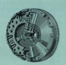
CLUTCHES - Big highcapacity coil-spring clutches, hydraulically actuated, harness the High Torque 401 and 478 engines in 13- and 14-inch sizes, respectively. Twin-plate clutches are available at extra cost in both sizes.
