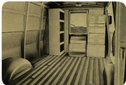
Routine delivery and service installation. Minimum bins and drawer space allow plenty of room for large bulky items.
