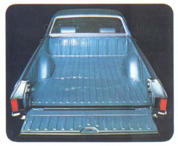
**CARGO BOX** is strong and spacious with room for objects more than six feet long. Reinforced steel floor and double sidewalls take the knocks on the inside without marring exterior beauty.
