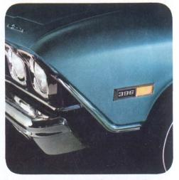
**SIDE MARKER LIGHTS** on the front only are amber colored. Lights are turned on when headlights are in operation.
