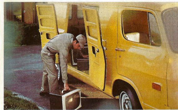
Right side cargo doors. Standard with 108" WB, available with 90" WB.
