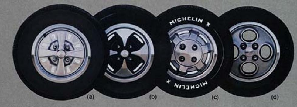
WHEELS AND TIRES. Handsome fully styled steel wheels (a) are standard on LN7. TR-type steel wheels (b) are included in the Sport Package. Cast aluminum spoke wheels (c) are included in the Grand
