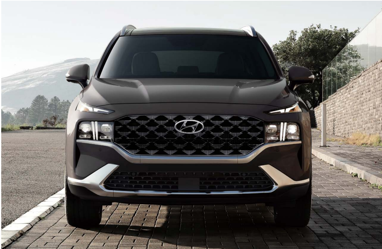
Standard LED headlights and LED daytime running lights with signature T-shaped design
