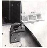
The cab is three-point mounted by means of highly efficient rubber-insulated pin and trun-nion-type hinged joints. One of the two front mountings is shown here. These long-life cab mountings prevent side movement and twisting.
