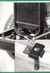
The radiator is mounted on large rubber pads between the radiator core support and the frame front crossmember which also carries the engine front mounting. This construction cushions the radiator against twists and stresses raused by operation over uneven ground.
