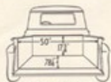
GMC 6½-F.T. PICKUP BODY For Models 101 and 101-8
