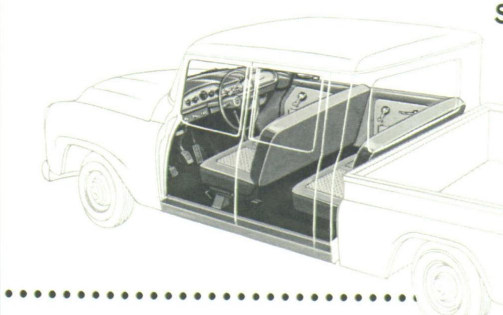
When 4 to 6-man crews with tools and equipment go on field assignments to hard-to-reach places, the combination of Model D-1100 (4x4) or D-1200 (4x4) chassis, 6-man Travelette cab and pickup or service-utility body is unmatched for convenience and economy. The Travelette has the same front area as the regular cab, plus a second full-width seat and two extra side doors for ease of entrance.
