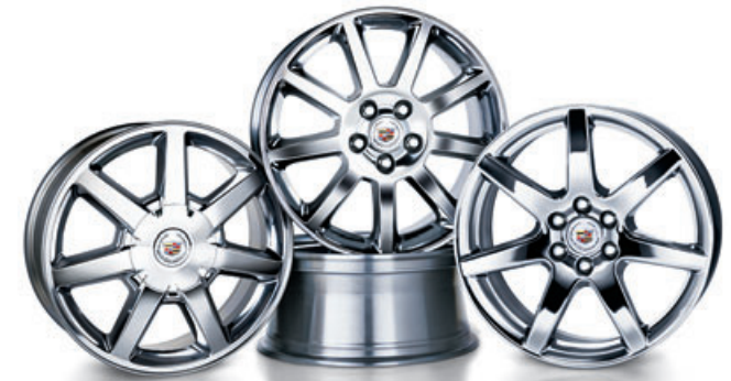
17-inch, cast-aluminum, polished, seven-spoke
