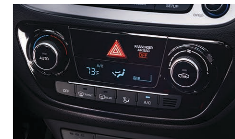
Automatic temperature control
